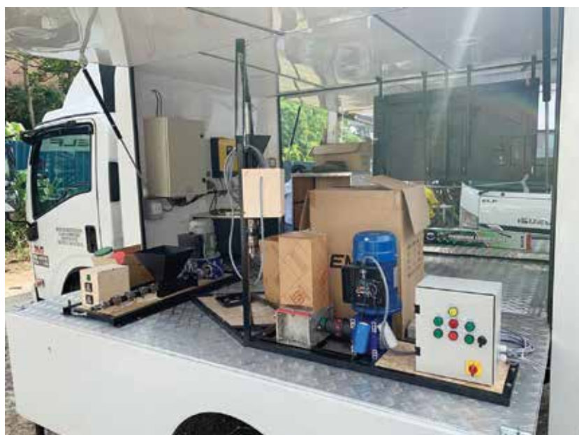
Simple recycling machines (from right to left: shredder, injection machine and extrusion machine) were fitted inside The Green Truck
