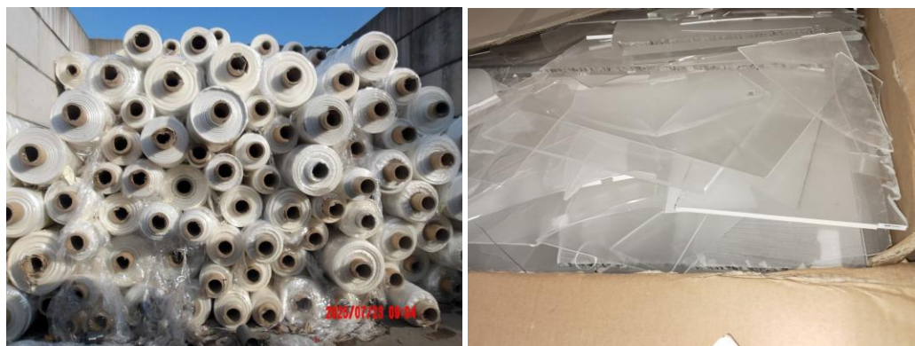
Photo caption: Clean and homogenous plastic feedstock imported by licensed recyclers: (left) industrial low-density polyethylene (LDPE) film in roll form and (right) polymethyl methacrylate (PMMA) acrylic sheets
